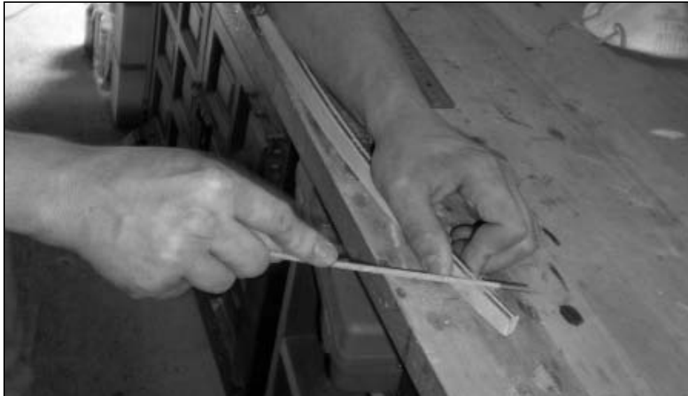
Picture 43: A chainsaw file has the perfect size for filing the temporary string grooves
