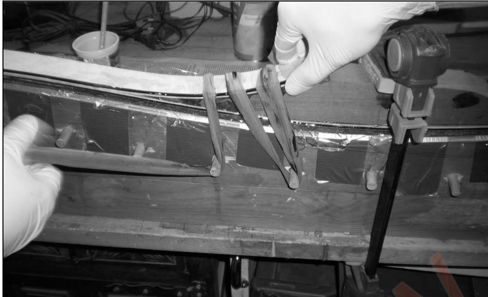
Picture 33: After fixing the riser piece in place with a c clamp we can start to laminate the rest of the bow. With rubber bands we press the lams into the form
