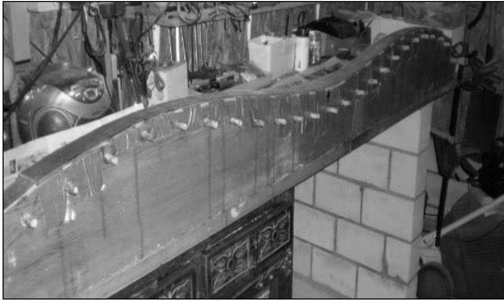
Picture 21: The form is ready for the glue up and we can start to build the bow
